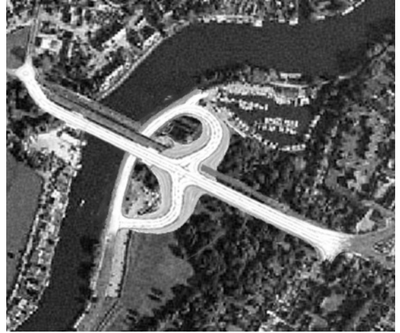
Surrey County Council's in-house design for a new permanent Walton Bridge, new viaduct and new 'clover leaf' junction at Cowey Sale
